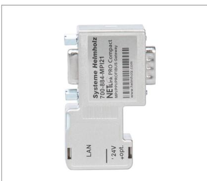
The current NETL ink® PRO Compact is especially suited for retrofits in existing systems and production lines. It is plugged directly into the port of the PROFIBUS/MPI participant and thus requires no additional space in the control cabinet. The NETL ink® receives the operating voltage through the active PROFIBUS device. In the case of passive participants in the network, the Ethernet gateway can be supplied with 24 V externally.
