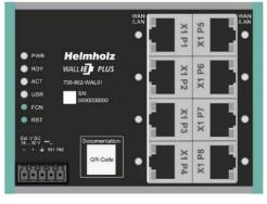
The configuration of the ports can be set in the "Device/ Ports Config" menu. All ports for LAN and all ports for WAN are switched to each other internally.
