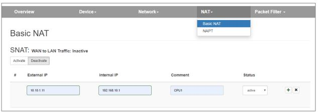
"External IP" is a free IP address from the WAN IP address range. This must not have been assigned to any other Ethernet station (in the WAN) yet! "Internal IP" is address assigned to physical device (the target device). WALL IE will map IP address according to NAT rule and forward packets from WAN to LAN and vice versa.
