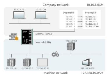
Broadcast traffic is generally filtered at the WALL IE, which means that the time behavior of the machine network is not impaired by the company network.
