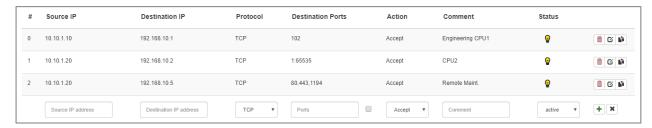
It is also possible to configure the access of several participants with one another. An IP range can be defined with a dash: "10.10.1.10-10.10.1.20". A list of IP addresses is indicated with commas: "10.10.1.10,10.10.1.15,10.10.1.20". IP subnet can be also declared using CIDR notation: "10.10.1.10/24".
