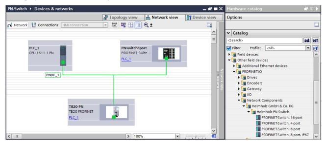
By calling up the object properties, you must assign the PROFINET switch a unique PROFINET name in the project and check the IP address for plausibility.
