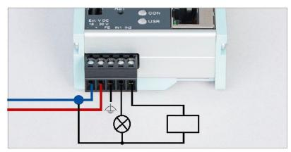
Example wiring of the outputs:
