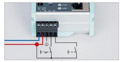
Example wiring of the inputs:
