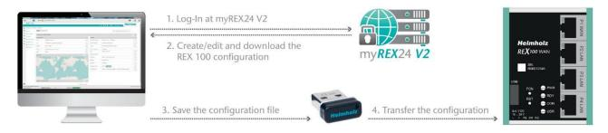
Ensure that the power supply is connected to the REX 100. Download the configuration file provided through the myREX24 portal to the FAT-formatted USB flash drive connected to your PC using the download symbol.
