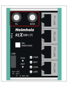
For the same reason, the second antenna should be mounted cross-polarized (rotated by 90° in relation to the main antenna).
