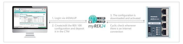
The Configuration Transfer Manager makes it possible to transfer the configuration to the REX 100 router once the router has established an Internet connection to the myREX24 portal.
