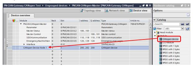
The parameters of the CANopen slave can be specified under the properties of the CANopen device entry. The device node ID of the CANopen slave must be set correctly.
