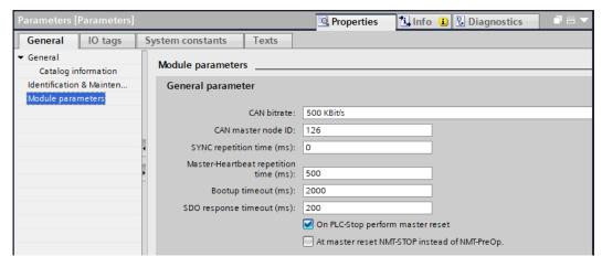
Set the CAN bit rate and the CAN master node ID. In some applications a SYNC telegram or heartbeat telegrams of the master is necessary for operation. The other "PN/CAN CO" slot entries do not contain any parameters.
