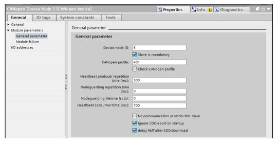
If the option "Slave is mandatory" is selected, all CANopen nodes on the CAN bus of the PN/CAN-Gateway are not switched to operational until this device is present and parameterized.
