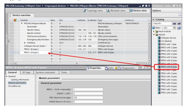
The order of the TPDO and RPDO entries in the configuration can be chosen arbitrarily. All TPDO and RPDO entries that follow a CANopen device entry belong exactly to this device.
