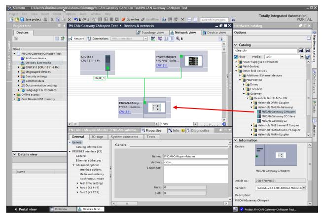
By calling the properties a unique PROFINET name should be assigned to the PN/CAN gateway and the IP address should be checked for plausibility.
