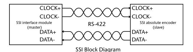
SSI provides several crucial advantages when compared to other interfaces for position measuring systems:
