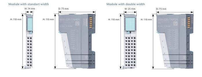
Communication Module W: 25 mm D: 73 mm H: 110 mm H: 110 mm Good - 400 - 74.31 Find the find
