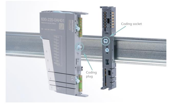
The coding plug and coding socket can each be in one of eight different positions. Each of these eight positions is factory-assigned to a specific type of module (digital in, digital out, analog in, analog out, power, etc.) from the TB20 I/O system. It is only possible to plug an electronic module into a base module if the positions of the coding plug and the positions of the coding socket match. Otherwise, the electronic module will be mechanically prevented from being plugged in.
