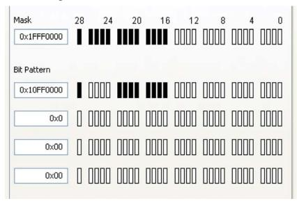
In order to receive any CAN telegrams the CAN identifier bits are first filtered with a mask and then compared with a predefined value (bitmap). If this comparison succeeds the CAN telegram is transferred to the other channel and forwarded to the CAN bus.
