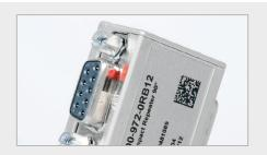
The PROFIBUS Compact Repeater is plugged directly onto the Sub-D socket of the PROFIBUS participant instead of the normal PROFIBUS device connector. It is fastened using the two screws above and underneath the socket.
