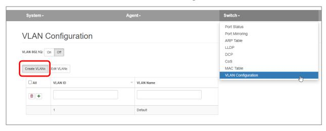
The VLAN ID can be set from 1-4095, the VLAN name is freely selectable.
