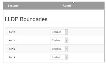
The form for querying and changing the LLDP settings is located under "LLDP" in the "Switch" menu.
