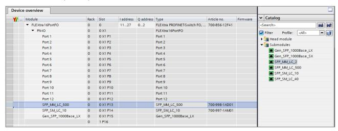
If the Helmholz SFP modules are configured, the FLEXtra PROFINET switch checks whether exactly the configured SFP module has been plugged into the specified port.
