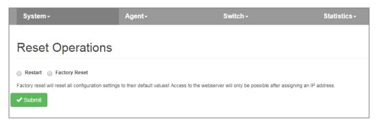
The restart of the device can also be triggered at any time also by pressing the "RST" button on the front panel of the device.
