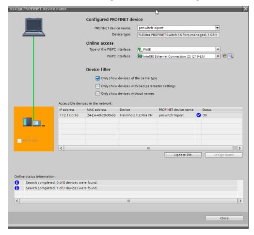
The clear identification of the FLEXtra PROFINET switch is ensured here by the MAC address of the device. The MAC address of the device can be found on the device front of the FLEXtra PROFINET switch.
