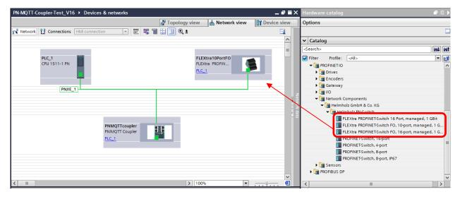
By calling up the object properties, you must give the FLEXtra PROFINET switch a unique PROFINET name in the project and check the IP address for plausibility.
