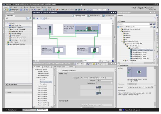
If the topology was specified in the configuration, the PROFINET name can also be assigned to neighboring devices in the event of a device swap. This makes it possible to detect and check the network topology and to "swap devices during operation" of connected PROFINET devices.
